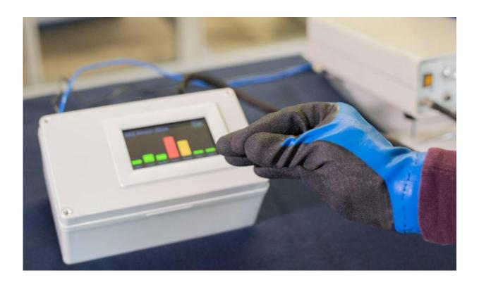
Measuring pressure with flexible pressure sensors. Credit: Fraunhofer ISC
