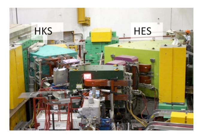
The magnetic spectrometers, HKS (High resolution Kaon Spectrometer) and HES (High resolution Electron spectrometer) used for the experiment. These spectrometers were constructed and tested in Japan and then shipped to JLab. Credit: Tohoku University
