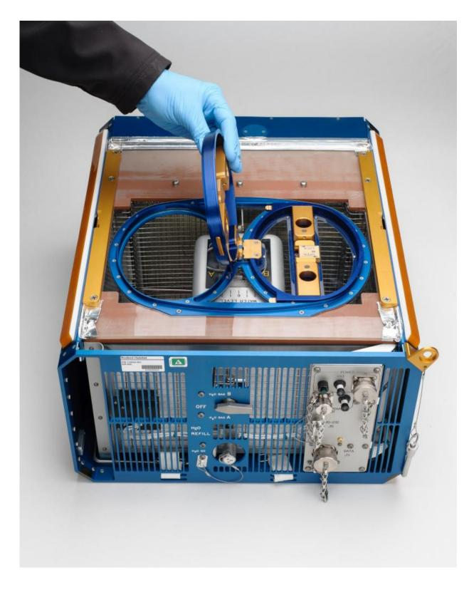
NASA's Rodent Habitat, shown here with one of the two access doors open, provides long-term housing for rodents aboard the International Space Station.
