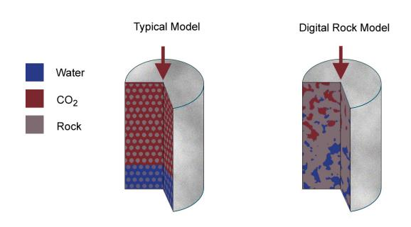
Chematic of a sandstone sample receiving CO2 injection, indicating the difference in detail in the simple typical model (left) and the more realistic digital rock model used in the study (right). The greater detail provided by the digital rock model can help to identify the relevant processes of CO2 movement and the rock's potential for CO2 storage in natural rock reservoirs. Credit: International Institute for Carbon-Neutral Energy Research (I2CNER), Kyushu University
