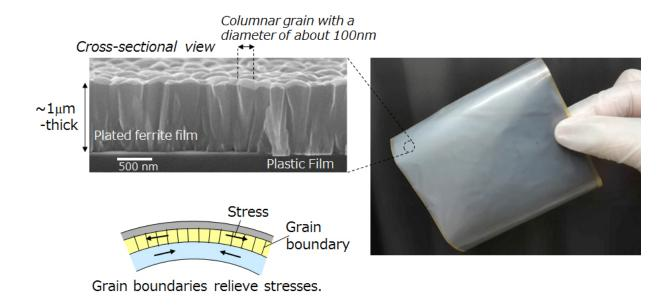
Devices with bending resistance and low heat treatment temperature achieved by new deposition technology.New deposition technology fabricates a fine ferrite film for spin Seebeck thermoelectric devices at 90°C, much lower than the 700°C used with the conventional method. Owing to the decrease in heat treatment temperature, elements can be created on the surface of plastic film, etc., and flexible devices of various shapes are created. Credit: NEC Corporation
