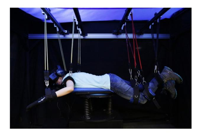
The Amphibian SCUBA diving simulator, a research project from the MIT Media Lab, lets users experience the underwater world through a high presence virtual reality system. The system includes a motion platform, Oculus Rift headmounted display, snorkel with sensors, leg-motion sensors, and gloves that enable motion detection, temperature simulation, and physical feedback of objects. Captured sensor data is fed into a processing unit that converts the users physical
