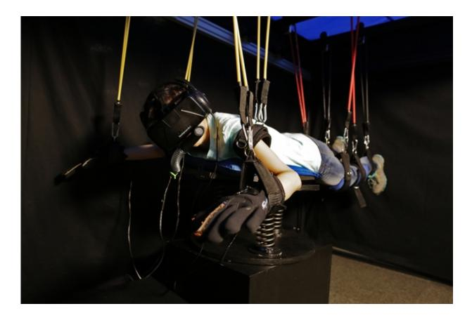
A user experiences the underwater world using Amphibian SCUBA diving simulator. The user is resting on a suspension system wearing Oculus Rift, a snorkel with breathing sensor, and gloves for motion detection. Credit: James Day
