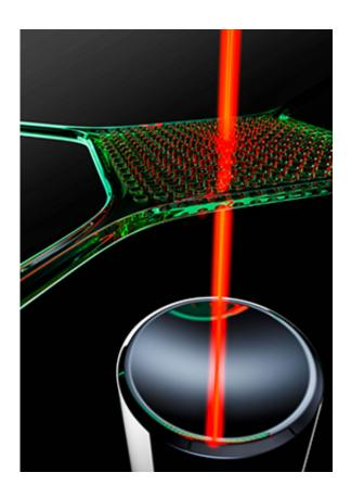
An artist's impression of the membrane coupled to a laser beam. The periodic pattern makes the device highly reflective, while the thin tethers allow for ultralow mechanical dissipation. Credit: Felix Fricke
