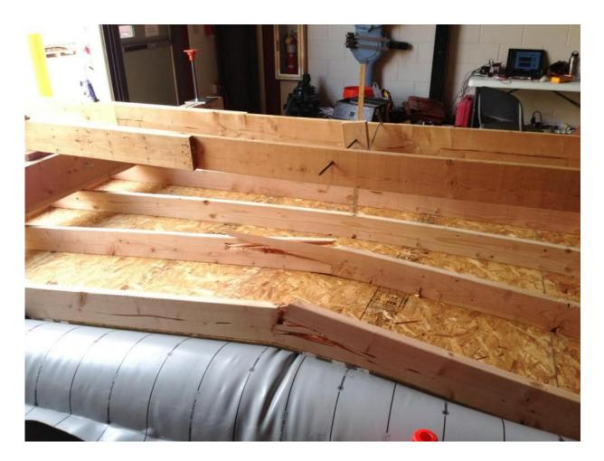
In a University of New Mexico lab, roofs were built and stressed to the breaking point to show the solar permitting community how strong they are. The tests were done by Sandia National Laboratories in partnership with UNM. Credit: Sandia National Laboratories
