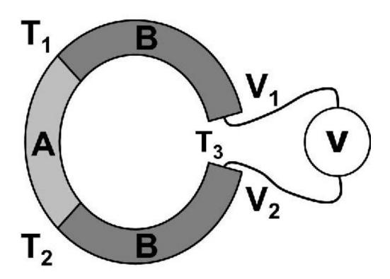
Determination of the Seebeck coefficient for a circuit composed of two dissimilar materials.
