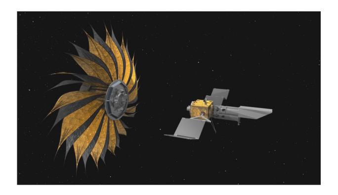
This illustration shows the prototype starshade, a giant structure designed to block the glare of stars so that future space telescopes can take pictures of planets.
