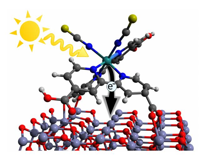
Illustration of the initial charge transfer step in a dye sensitized solar cell. A photon from the sun is absorbed and excites the dye molecule. Subsequently, an electron can is injected into the ZnO-Layer where it can be trapped by so called interface-states. Credit: HZB/Mario Borgwardt
