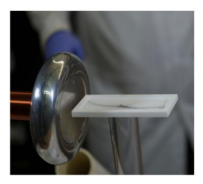
Nanotube wires self-assemble under the influence of a directed electric field from the Tesla coil. Credit: Jeff Fitlow
