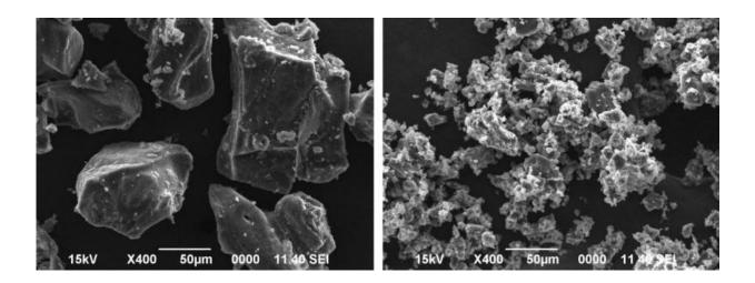
Chunks of this sodium-based compound (Na2B12H12) (left) would function well in a battery only at elevated temperatures, but when they are milled into far smaller pieces (right), they can potentially perform even in extreme cold, making them even more promising as the basis for safer, cheaper rechargeables. Credit: Tohoku University, Japan
