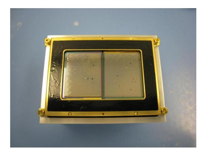
This kilopixel detector array developed by Goddard technologist Christine Jhabvala is similar to the four arrays flying on the PIPER mission. Each array contains 1,280 pixels, each about 1-milimeter square, composed of a membrane of silicon 1 micrometer in thickness. (Photo Credit: Christine Jhabvala/NASA) Credit: NASA/C. Jhabvala
