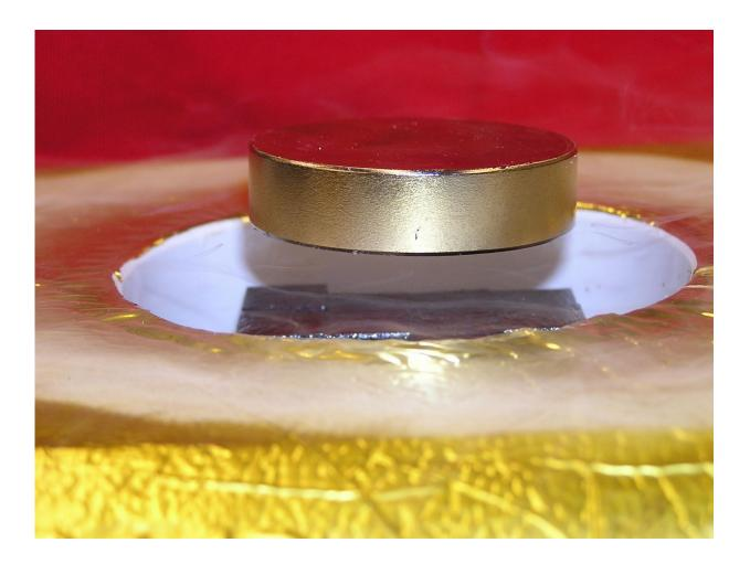
This image of a magnet levitated over a high-temperature superconductor array shows rectangular TFMs (black) levitating a heavy ferromagnet (silver) above a container of liquid nitrogen. Credit: Weinstein/University of Houston
