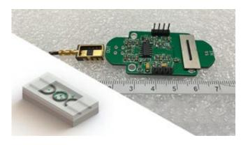
A schematic (left) and photograph (right) of a photonic dew point temperature sensor developed by Ji Fang Tao and co-workers, which works by detecting changes in the refraction of light as water molecules condense onto the device. Credit: (left) © 2015 IEEE. Reprinted, with permission, from Ref 1. (right) © 2016 A\*STAR Institute of Microelectronics
