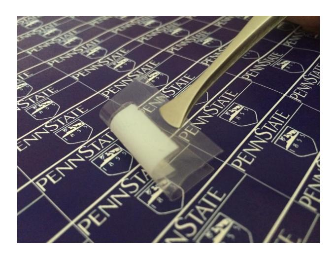
Nanowire array electocaloric fabric placed on flexible substrate is flexible. Credit: Qing Wang, Penn State
