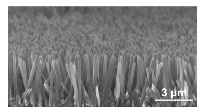
The tiny wires of the nanowire array form on a template so they are uniform. Credit: Qing Wang, Penn State
