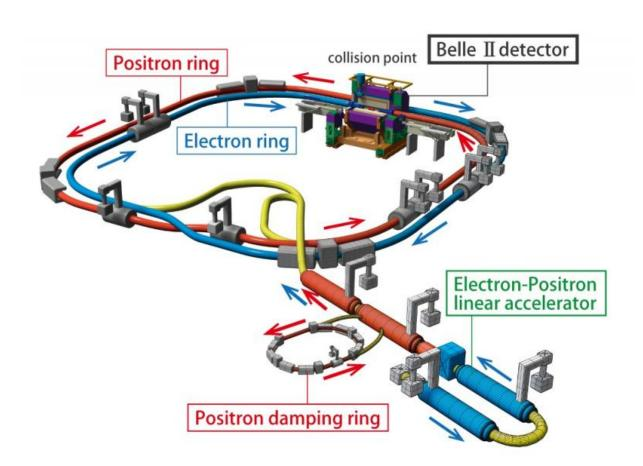
Plan of the SuperKEKB accelerator with the Belle-II detector. Credit: KEK
