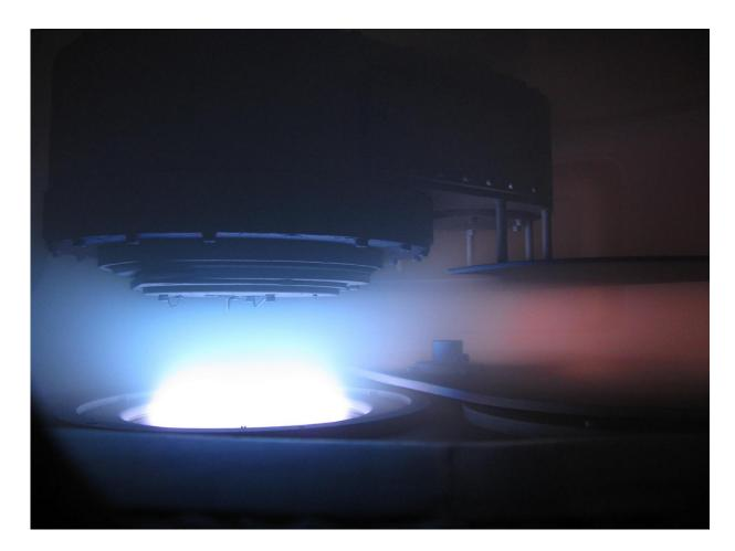
View inside vacuum chamber during the coating process. Credit: © Photo Fraunhofer IWM
