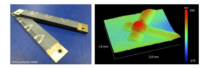
Sealing bars fitted with thin-film sensors (left). White light interferometer image of a measuring point with conducting tracks approx. 250 nm thick and 600  $\mu$ m wide (right). Credit: © Photo Fraunhofer IWM
