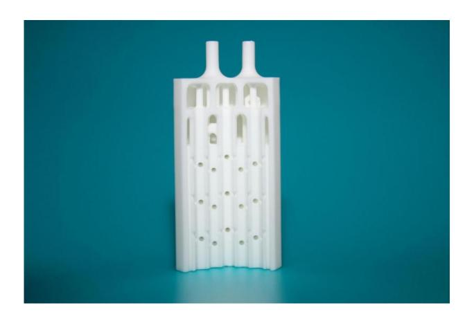
Cut through a ceramic microreactor which was manufactured additively: the complex channels as well as the fluidic connections at the top were printed together with the whole component.
