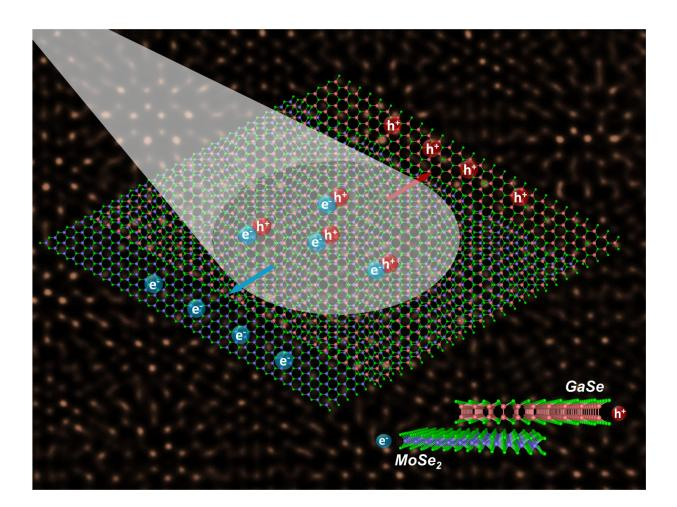
Light drives the migration of charge carriers (electrons and holes) at the juncture between semiconductors with mismatched crystal lattices. These heterostructures hold promise for advancing optoelectronics and exploring new physics. The schematic's background is a scanning transmission electron microscope image showing the bilayer in atomic-scale resolution. Credit: Oak Ridge National Laboratory, US Dept. of Energy. Image by Xufan Li and Chris Rouleau
