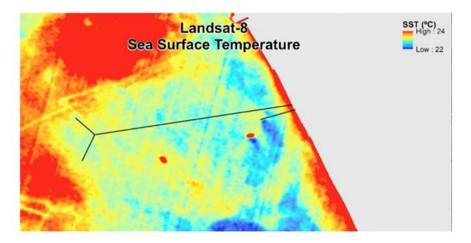
Landsat-8 image of water temperature in Santa Monica Bay on Oct. 10, 2015, during the diversion. Black lines mark the short active pipe and long inactive pipe. Treated wastewater is visible as an area of cooler water flowing south from the active pipe. The two red dots are ships. Credit: NASA/USGS
