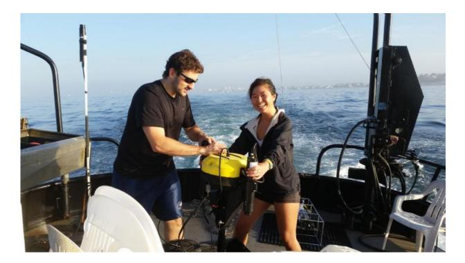
During the wastewater diversion monitoring, JPL scientists Cedric Fichot and Rebecca Trinh used an in-water instrument called an optical profiler to gain information on chlorophyll and other organic matter in the water. Credit: NASA/JPL-Caltech
