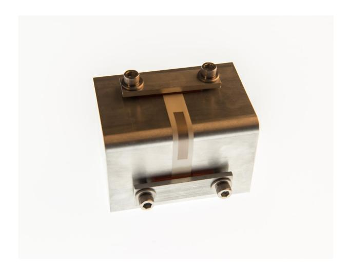
This image shows a flat liquid crystal polymer (LCP) strip containing gold traces or wires that were printed with a technique called aerosol jet printing. The traces are 60 microns wide, smaller than a human hair. Credit: NASA/W. Hrybyk
