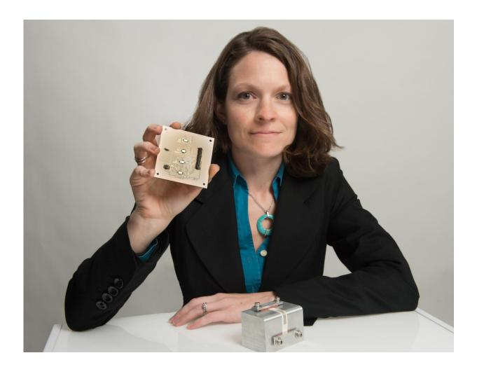
Goddard technologist Beth Paquette holds a 3-inch-by-3-inch ceramic board with four radiation-hardened digital-to-analog converter chips (in the middle of the board). She created the circuitry using a 3-D printing technique using silver ink. Credit: NASA/W. Hrybyk
