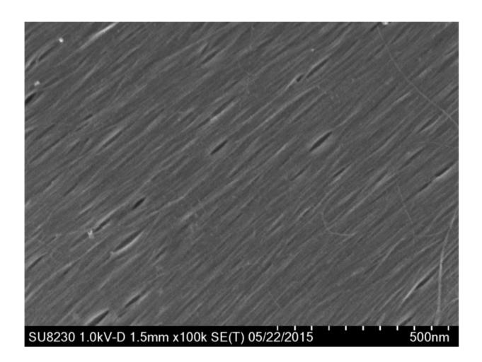
A scanning electron microscope image shows highly aligned and closely packed carbon nanotubes gathered into a film by researchers at Rice University. Credit: Kono Lab/Rice University
