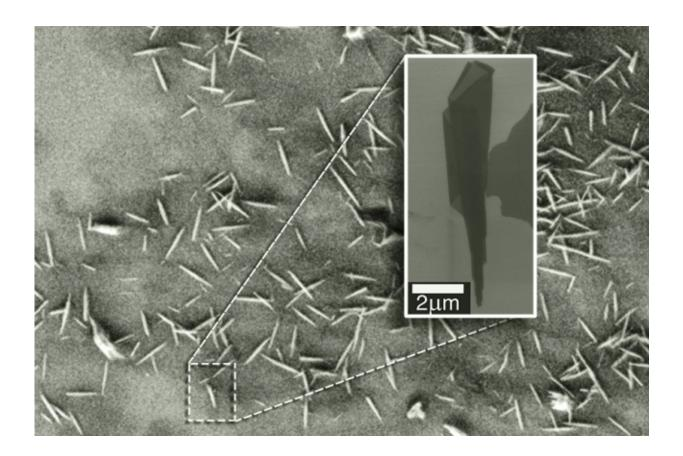
An electron microscopy image shows many examples of nanoscrolls. The insert zooms in on a single nanoscroll and reveals its conical nature.
