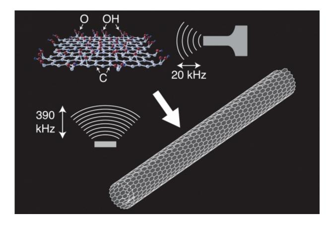
This sketch illustrates how a nanoscroll forms from a graphene oxide flake as a result of ultrasonic irradiation.
