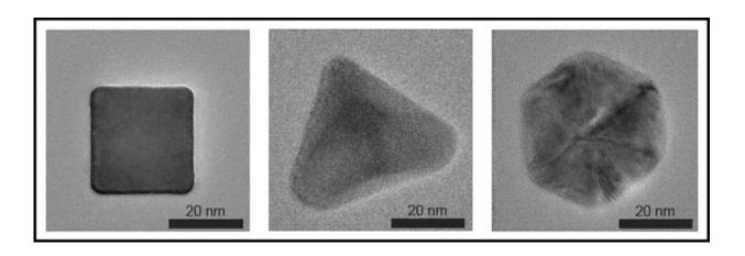
Stanford engineers studying the structures of phase-changing nanoparticles have found that shape matters. Materials composed of cubes and pyramids, for instance, may yield more efficient batteries than those made of icosahedra. Credit: Dionne Group
