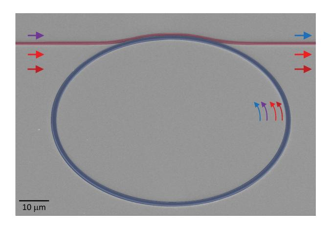
False-colored scanning electron micrograph of the nanophotonic frequency converter, consisting of a ring-shaped resonator (shaded blue) into which light is injected using a waveguide (shaded red). The input signal, depicted as a purple arrow, is converted to a new frequency (blue arrow) through the application of two pump lasers (light and dark red arrows). Credit: K. Srinivasan et al./NIST
