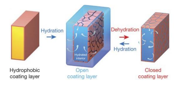
A hydrophobic coating layer provides a self-controlled mechanism for water conservation using nanometre-sized cracks (nanocracks) tuned by membrane swelling behaviour in response to external humidity conditions, which act as nanovalves. Credit: Chi Hoon Park et al. *Nature* (2016). DOI: 10.1038/nature17634
