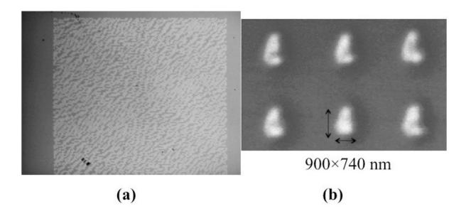
Image composed of nano-magnetic pixels. (a) A 256×256-pixel 1 micrometer-pitch image obtained via polarization microscopy and (b) a 3×2-pixel 2.5-?m-pitch image obtained via magnetic force microscopy. Credit: (c) Toyohashi University Of Technology
