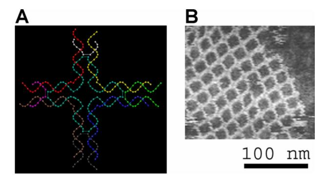
At left, the design of a single tile of a nanogrid made of DNA; at right, the grid as viewed by an atomic force microscope. Credit: Strong, 2004, CC BY
