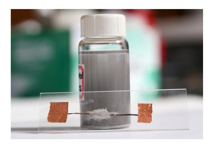
The vial contains liquid-metal particles suspended in ethanol. The particles were used to demonstrate heat-free soldering. Credit: Christopher Gannon/Iowa State University
