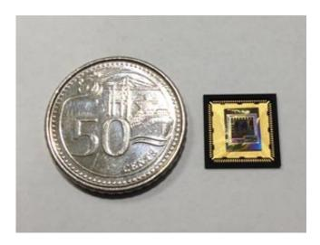
A test chip for a sensor node processor based on cognitive sensing technology. A 50-cent coin has been placed next to the chip for size comparison. Credit: A\*STAR Institute of Microelectronics
