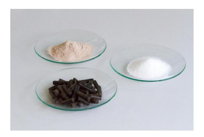
With the BioEcoSim process, livestock manure can be converted into valuable phosphorus fertilizers (rear), nitrogen fertilizers (right) and soil conditioners (front).
