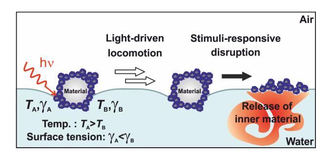
Scheme illustrating the light-driven delivery of material using liquid marbles (LMs). Credit: © WILEY-VCH (2016)
