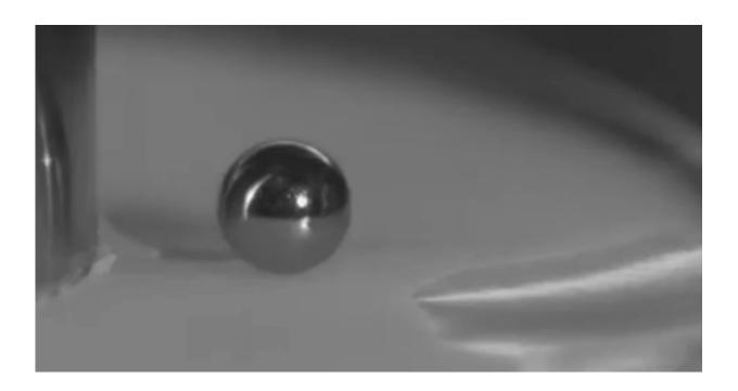
The attached image shows how a small steel sphere sits on a shear-jammed suspension just as it would on an ordinary solid. Removing the shear switches the suspension back to its liquid-like state and the sphere would sink. Credit: University of Southampton
