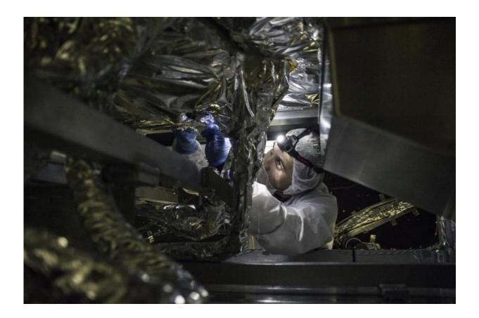
Technician Andrew Peterson installs thermal blankets to the underside of the James Webb Space Telescope test model. Credit: NASA/Goddard/Desiree Stover
