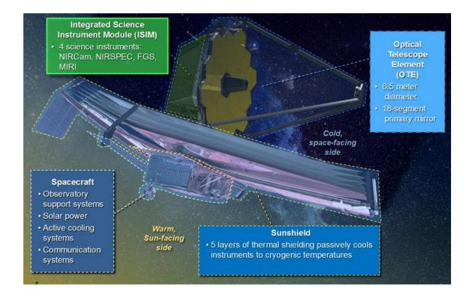
This graphic shows how the modules of the James Webb Space Telescope connect in the fully deployed observatory. Credit: NASA/Goddard/Paul Geithner
