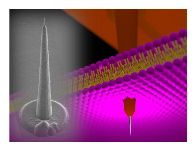
120-µm-height 'nanotower' electrode is punching a cell membrane. Silicon growth technology and three-dimensional nano/microfabrication techniques realize such high-aspect-ratio intracellular electrodes. Credit: (c) Toyohashi University Of Technology.
