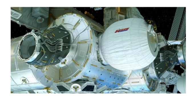
A render of the BEAM attached to the International Space Station. Credit: Bigelow Aerospace
