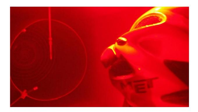
In the laboratory, Empa researchers simulate sunlight and airflow using infra-red light and a fan.
