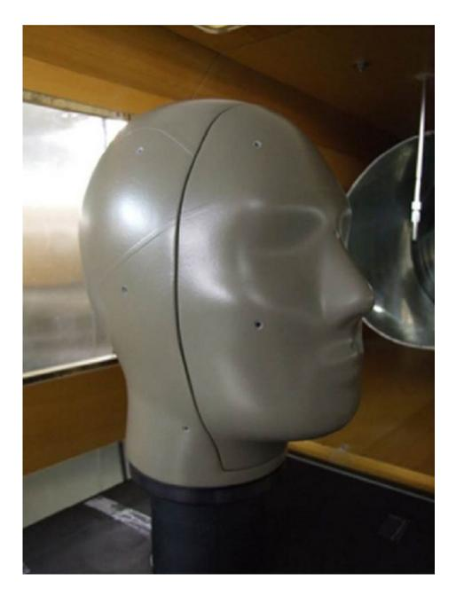
The boundary lines on the surface indicate the division of the head model into nine zones. The openings represent artificial pores through which the model can give off moisture, or "sweat."
