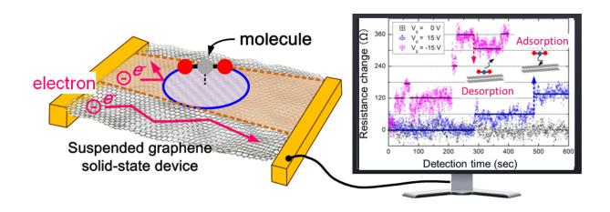
A diagram of a graphene single molecular sensor (left) and the observed signal showing successful detection of single CO2 molecule adsorption / desorption events. Credit: University of Southampton
