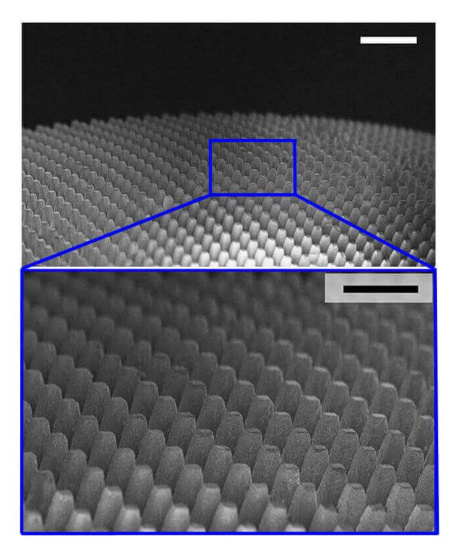
The field of tiny mirrors in the artificial eye was inspired by cup-shaped cells in the eyes of elephantnosed fish that help them see dark, murky water. Credit: Hongrui Jiang
