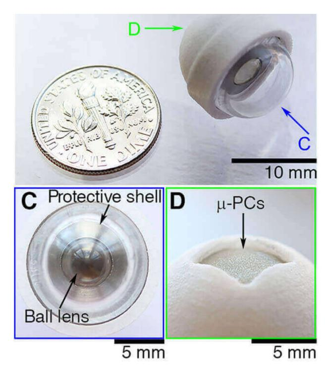
The ball-shaped, fingertip-sized artificial eye uses thousands of mirrors and a domed shape (seen in image D) to concentrate scant light. Credit: Hongrui Jiang
