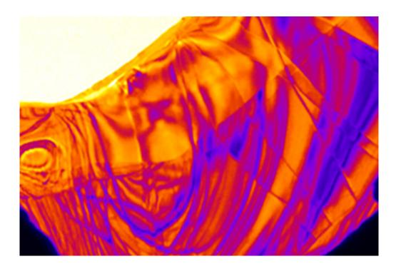
This is a false-colored ultrafast electron microscope (UEM) snapshot of a thin semiconducting crystal. The image was captured with an extremely fast shutter lasting only a few hundred femtoseconds (a millionth of a billionth of a second). Credit: College of Science and Engineering
