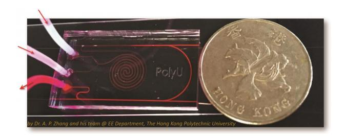
Fiber optic biosensor-integrated microfluidic chip detects glucose levels from droplets of sweat. Credit: Dr. A. P. Zhang and team, The Hong Kong Polytechnic University
