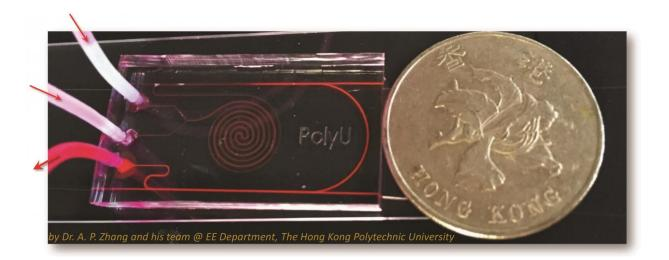
Fiber optic biosensor-integrated microfluidic chip detects glucose levels from droplets of sweat. Credit: Dr. A. P. Zhang and team, The Hong Kong Polytechnic University
