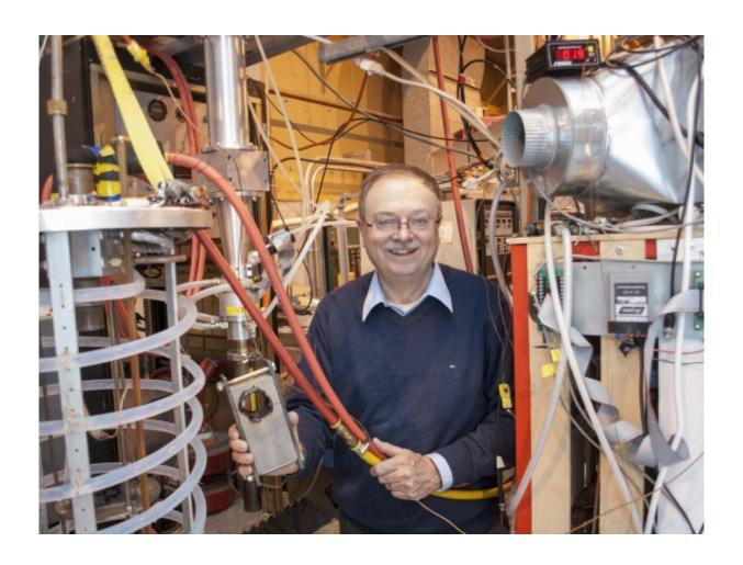
In one hand, senior research engineer Paul Woskov holds orange water cooling lines that lead to the rock test chamber (left foreground), and in the other the result of drilling rock with a gyrotron beam. Credit: Paul Rivenberg
