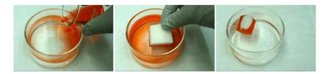
Water is contaminated with silicone oil (dyed red) and the newly developed sponge material is swept over the surface to absorb the oil layer; the oil-saturated sponge floats in the dish and can easily be picked up out of the clean water. Credit: Justin Weibel
