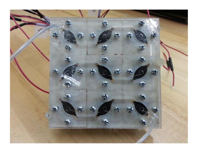
Nine biological-solar (bio-solar) cells connected into a bio-solar panel. The panel has generated the most wattage of any existing small-scale bio-solar cells - 5.59 microwatts Credit: Seokheun "Sean" Choi
