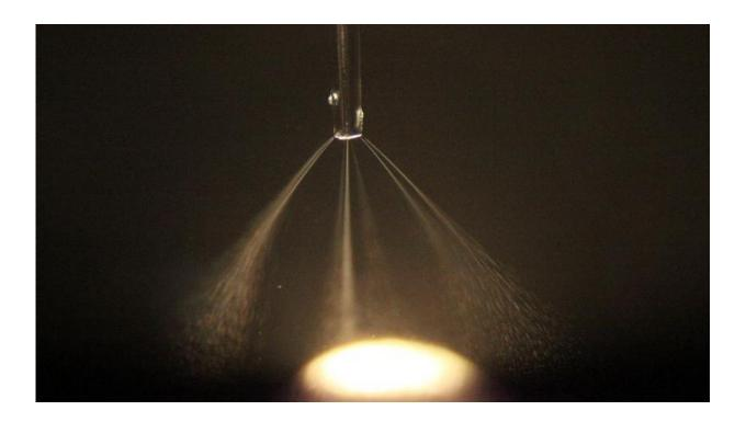
For the development of artificial muscles, the Empa scientists experimented with alternating current electrospraying
