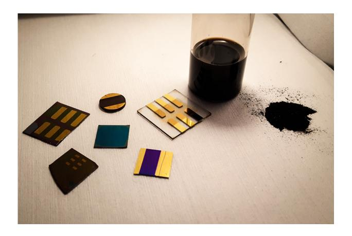
"When you look at coal as a material, and not just as something to burn, the chemistry is extremely rich," says Jeffrey Grossman. In this photo, a sample of pulverized coal (right) is shown with several test devices made from coal by the MIT researchers. Credit: Photo courtesy of the researchers
