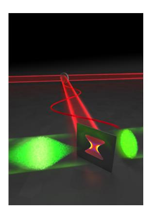
Pulses of electrons (green, coming from the left) impinge on a micro-structured antenna which is powered by laser-generated terahertz radiation (red). The interaction compresses the duration of the electron pulses to a few femtoseconds. Credit: Christian Hackenberger
