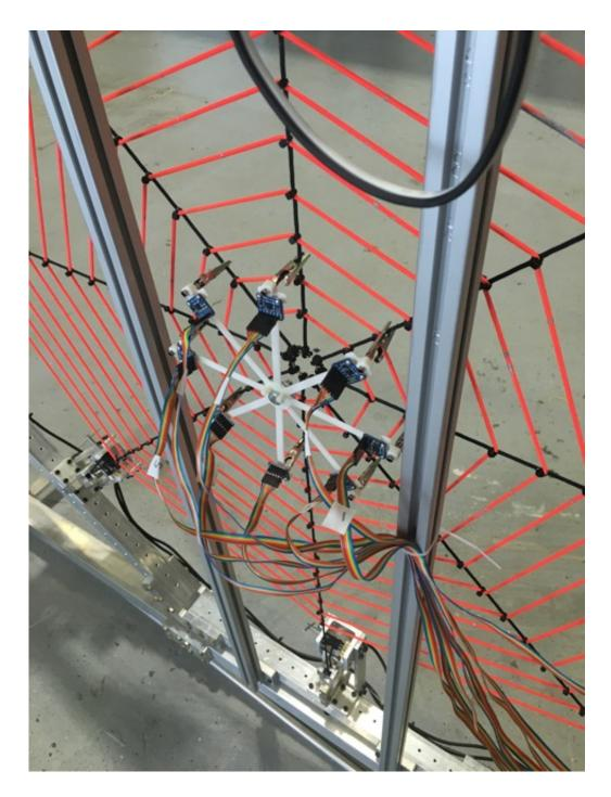
An artificial spider web, engineered by Ross Hatton of Oregon State University. With NSF funding, Hatton has teamed up with a spider biologist to probe the physics of spider webs. This artificial structure allows Hatton to precisely measure vibrations in the spider web, feeding into a computational model that will then be tested with real-life spiders. Credit: Andrew Otto, Oregon State University
